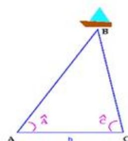
Up till now, we have seen how the science of angles, by comparing proportions, can be very useful. Now, with triangulation, one can go “beyond” angles themselves and, on the basis of the properties of triangles, “discover” distances otherwise unknown to simple sense perception.
