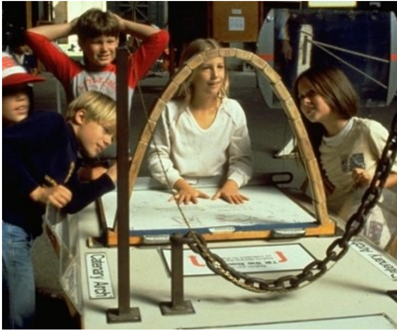
Figure 11. Constructing a vault without centering: a children's game when one uses the catenary!
