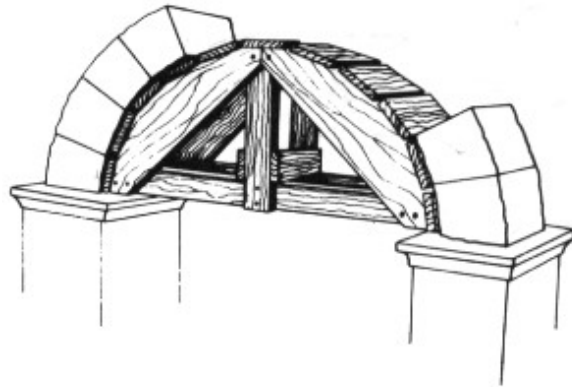
Figure 5. “Falsework” was used to construct both the circular and the pointed arch..
