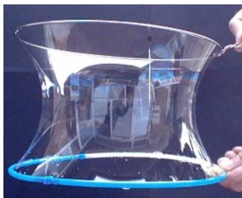
Figure A. The catenary curve generated by plunging two parallel iron-wire circles in liquid soap diluted in water forms the “optimal” volume of a catenoid.
